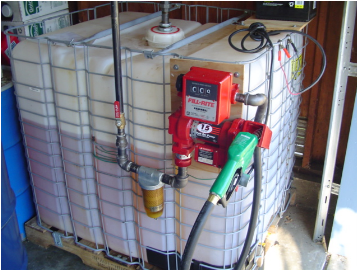
275 gallon plastic tote on pallet, 40"x48"x48"; 15 GPM DC pump w/meter, filter & auto shut off nozzle; battery
